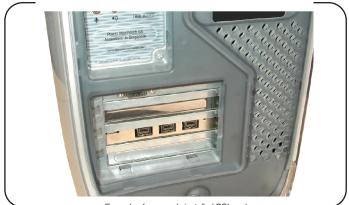
Example of a properly installed PCI card.
